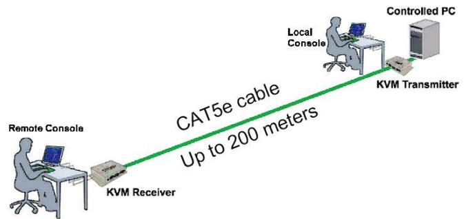
The Kit effectively extends PC KVM (Keyboard, Video and Mouse) control to the Console Receiver and also provides for convenient dual access; in addition to the Receiver console access, you can also connect a monitor/ keyboard/ mouse at the Transmitter site for local PC access.
